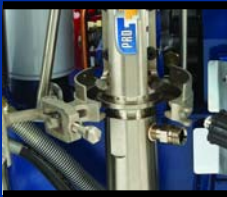
ProConnect™ system OPEN with pump in.
